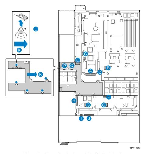
Figure 43. Removing the Power Distribution Board
